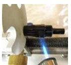
Heat shaft adapter with a butane torch or heat gun for a period of 20-30 seconds. BE CAREFUL IT WILL BE RED HOT!
