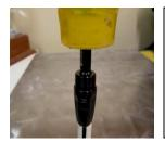
Place the butt end of the shaft on the ground and tap the end of the shaft adapter with a rubber mallet as shown. This ensures that the shaft is fully seated. Review your installation alignment and set aside to dry.
