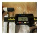
After you have trimmed the shaft, measure 0.950" from the end of the tip section and mark with a permanent marker. Wrap a piece of masking tape just above this mark.
