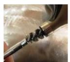
Remove the hosel adapter installation tool and the hosel adapter assembly with the protected hand and place aside to cool down.
