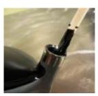
Prepare a mixture of high strength shafting epoxy and coat the inside diameter of the club head hosel. <u>DO NOT COAT THE HOSEL ADAPTER AT</u> THIS TIME!
