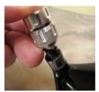
Slip the nut over the hosel adapter and re-insert tool. Apply pressure against the top of the tool while pulling the nut upward until it stops. Maintain this position and coat the outside of the hosel adapter with epoxy.
