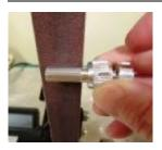
Slip the nut over the hosel adapter and insert the installation tool into the hosel adapter. Power the sander on and hold the nut in place while rotating the tool to lightly sand the outside of the hosel adapter as shown.
