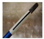
Place a vertical mark in the twelve o'clock installation position of the shaft.
