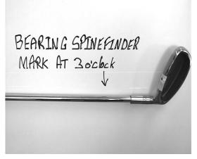
4 - Position the spine mark at 3 o'clock. Positioning the mark away from the target installs the shaft's natural curvature toward the target. In my opinion, this orientation promotes a freer release of the shaft through impact by reducing compression forces on the target side of the shaft and reducing tension forces on the backside of the shaft. A Stable Bending Plane is generally located within a few degrees of the spine mark.
