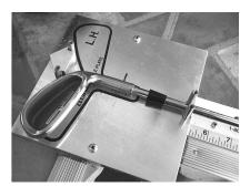
5 - Slide the ferrule onto the shaft and insert the shaft into the clubhead.
