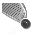
NOTE - If the swingweight is higher than desired, 2-3 grams can be removed by deep drilling the hosel. Use a smaller-than-bore drill bit, and ensure the bit does not penetrate the hosel as it nears the offset.
