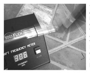
7 - Release and observe the dot orientation relative to the horizontal laser beam. Reorient the shaft and clubhead as necessary and repeat this test until the shaft moves straight back and forth with no off-plane oscillation to achieve the Stable Bending Plane. Most of my clients comment how every club feels and hits alike once the Stable Bending Plane is aligned perfectly perpendicular to the clubface.
