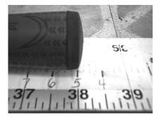
6 - Verify the total club length is *exactly* as desired. If necessary, retrim the shaft to achieve the *exact* length desired, then slide the ferrule down to the hosel.
