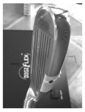
5 - Align the clubhead using the vertical laser and apply and mark a small piece of masking tape at the horizontal laser beam.
