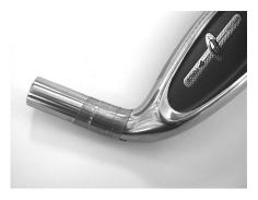
NOTE - If the swingweight is lower than desired, wrap lead tape around the hosel exterior until the target swingweight is achieved.
