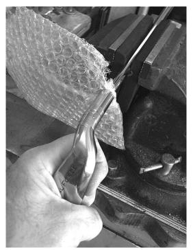
1 – Use a piece of bubble-wrap to force fit the lowest-frequency shaft into the longest clubhead. To obtain an accurate shaft frequency, it is imperative the clubhead fit tightly to the shaft. Layer the bubble wrap to ensure a tight fit, and if necessary use a hammer and butt plug to seat the shaft in the clubhead.
