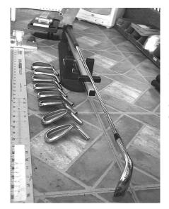
7 - Check the swingweight. It should be  $\frac{1}{2}$ -point lower than desired for final assembly. (The weight of the epoxy during final assembly will add the final  $\frac{1}{2}$ -point.)
