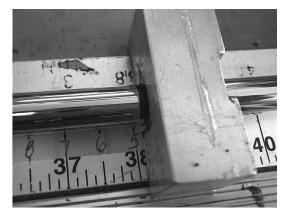
2 - Position the spine mark away from the target, and mark the shaft to the desired playing length.
