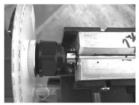
3 - Clamp the shaft in a frequency meter at the playing length mark
